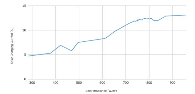
FIGURE 7: SOLAR CHARGING CURRENT VS SOLAR IRRADIANCE
