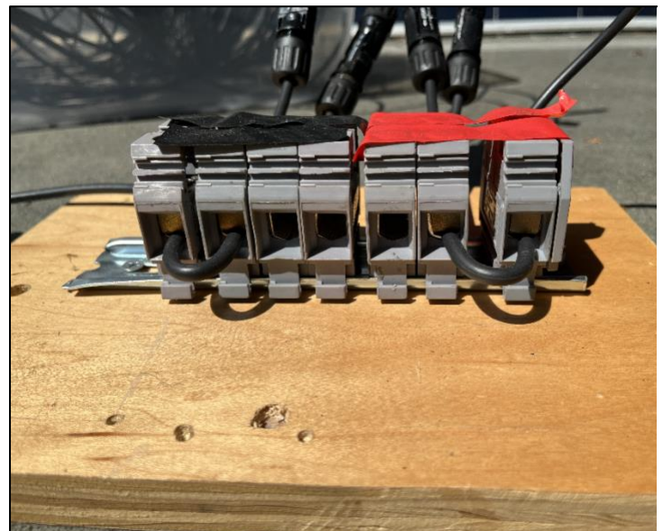
Figure 7. Parallel adapter for PV array circuits that have two parallel strands.
