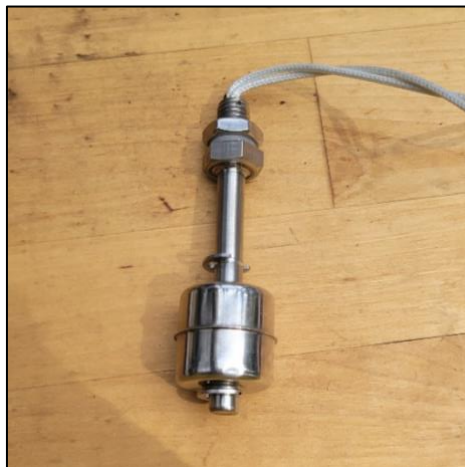
Figure 3: Example of a generic water level sensor (this one is a float switch device).
