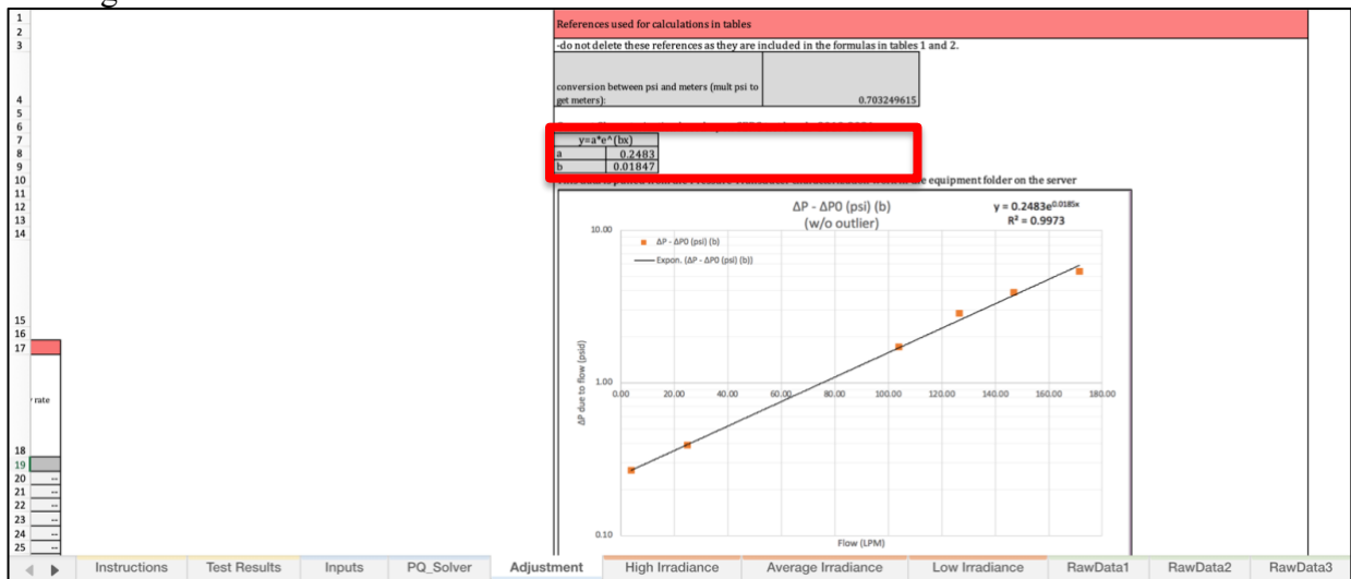
Figure 35. IrradianceData spreadsheet Adjustment tab, where the coefficient and slope from last plot made should be entered (in the red rectangle).
