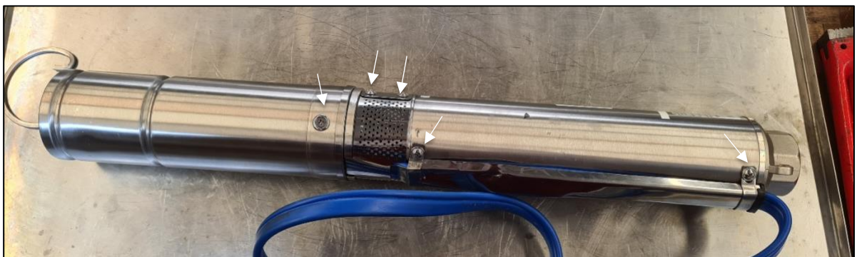
Figure 3: External screws on a submersible water pump.
