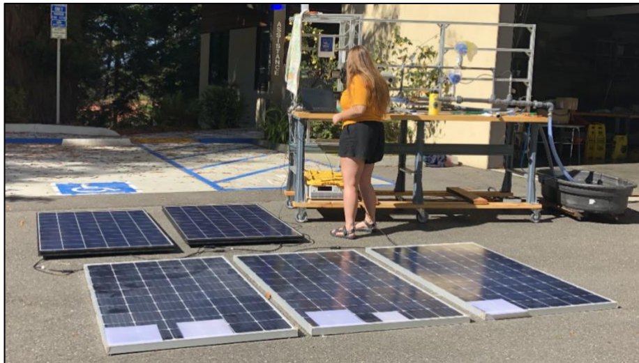
Figure 10. One tester at the test bench laptop to record results; another tester in charge of the PV array shading.
