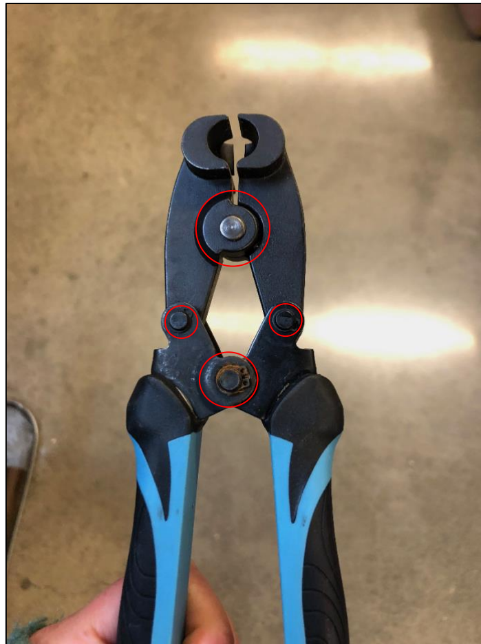
Figure 4. Crimper and red circles indicating where it should be annually oiled.
