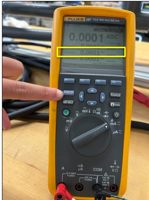
Figure 25. HOLD button on the Fluke DMM and the average measured value over the time interval in the yellow rectangle.
