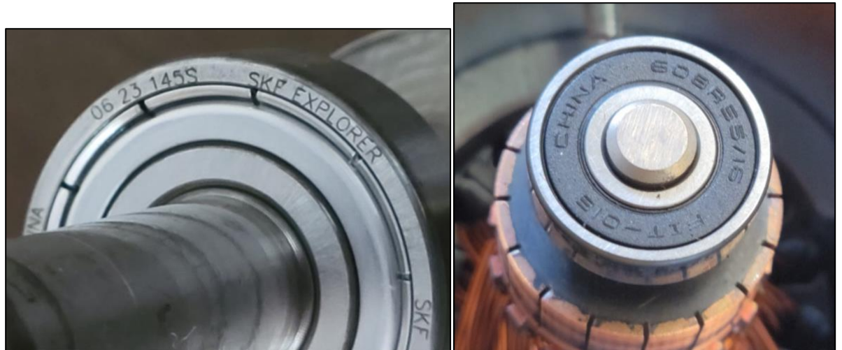
Figure 15: Example of close-up pictures documenting the brand and model number printed on the bearing.
