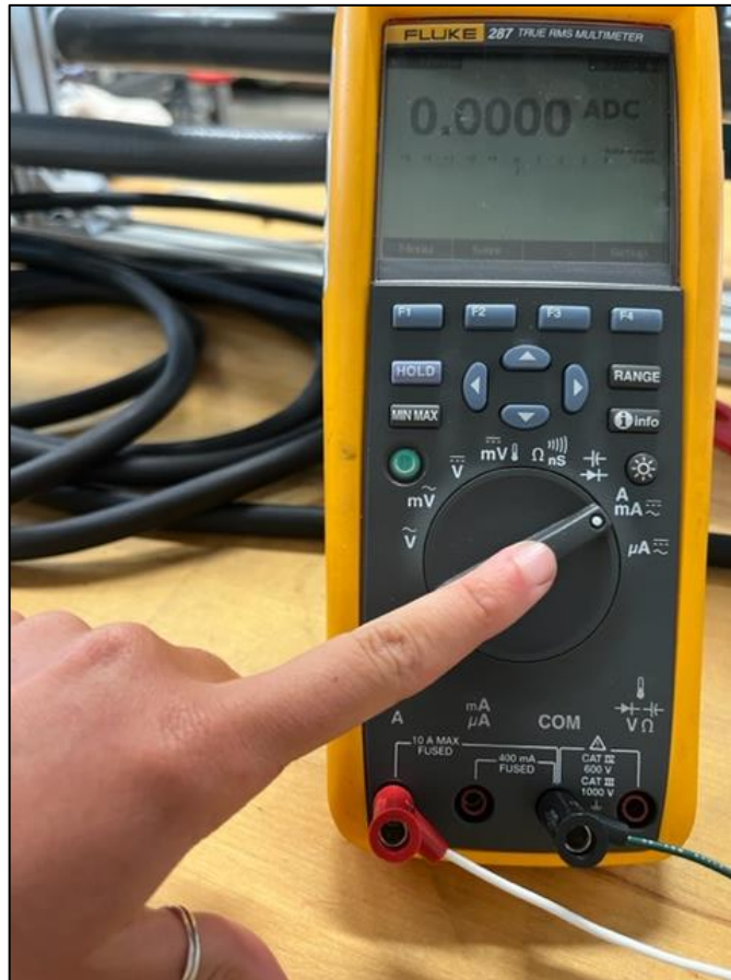
Figure 23. Fluke DMM in the mA setting with banana plug adapters already plugged in.
