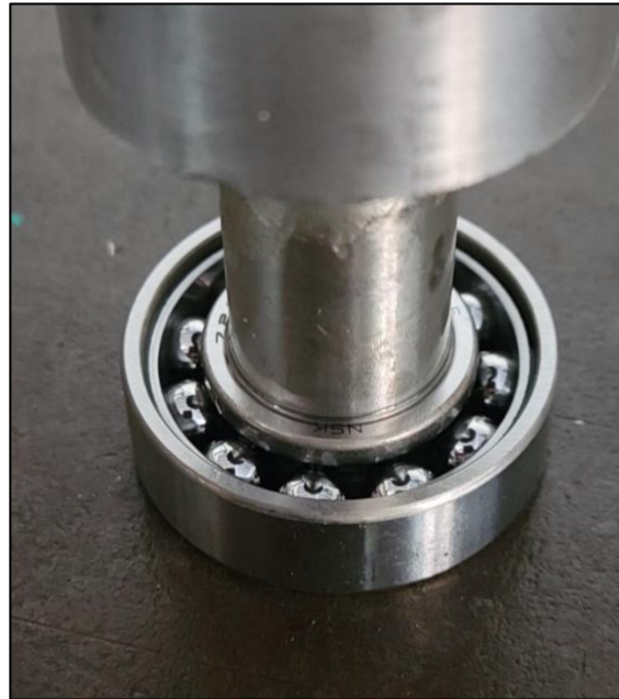
Figure 16: Example of an unsealed bearing.
