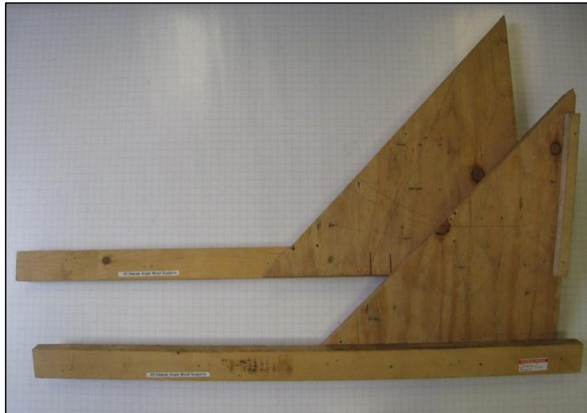
Figure 10. Custom angled wood cuts for strain relief.
