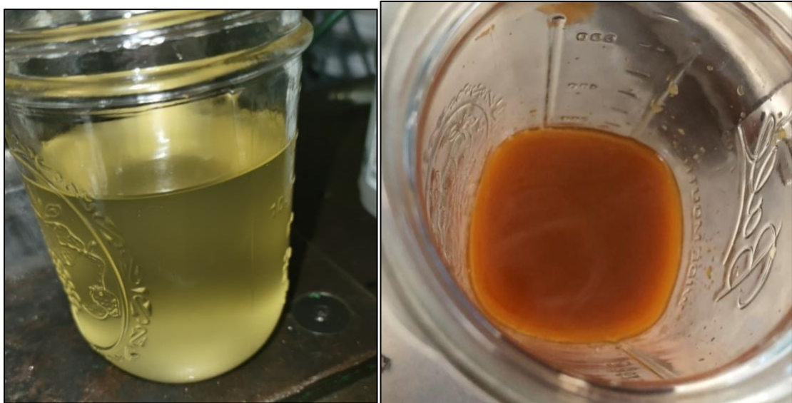
Figure 9: Example of clear and good quality oil (left). Example of debris and rust in motor oil (right).
