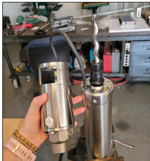
Figure 23: Example of a submersible helical rotor pump.
