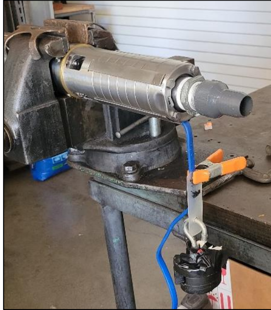
Figure 6: Pump set up for 90° angle.
