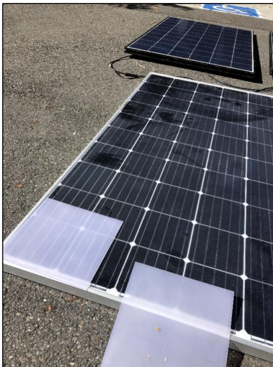
Figure 9. Semi-clear plastic squares to provide some coverage to PV modules to reduce and control power input.
