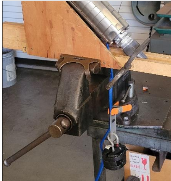
Figure 5: Pump cable set up in the strain relief apparatus for 45° angle testing.
