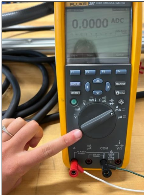
Figure 18. Fluke DMM on mA setting with the banana plug adapters plugged into the COM and 10A fuse ports (note the 400mA fuse port should be used in place of the 10A fuse if the mA reading using the 10A fuse is <math><400\text{mA}</math>).
