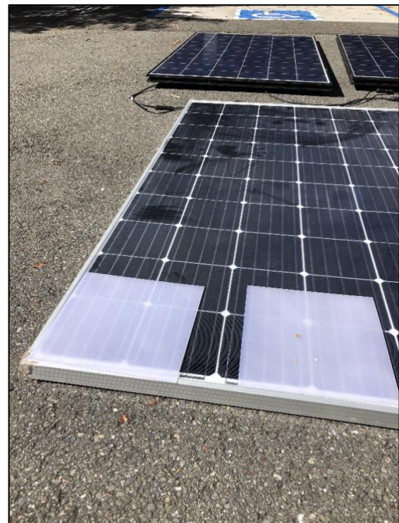
Figure 9. Semi-clear plastic squares to provide some coverage to PV modules to reduce and control power input.
