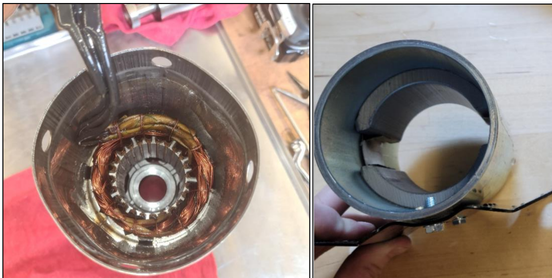
Figure 14: Two different stator types: one that is a part of an induction (AC) motor (left) and another that is a part of a DC motor (right).
