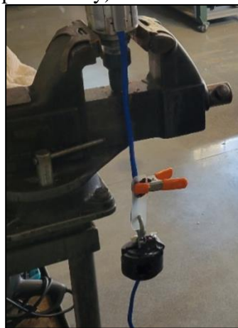
Figure 4: SWP cable in the vice grip for the 0° configuration.
