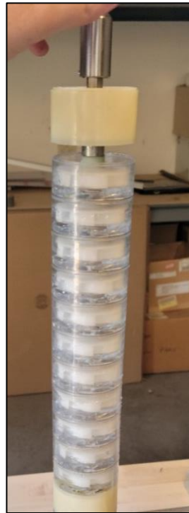
Figure 22: Example of submersible centrifugal pump.
