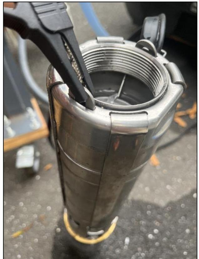
**Figure 15. Alligator clip connected to the pump body on one side; the other side, connected to the extender cable that connects to the Chroma grounding screw terminal box.**
