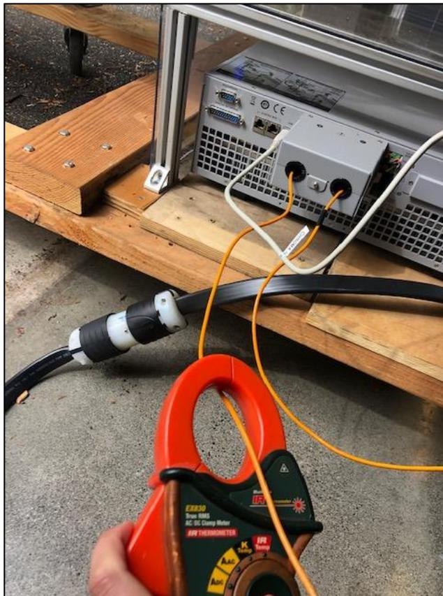
**Figure 5. Clamp meter around output lead of Chroma**
