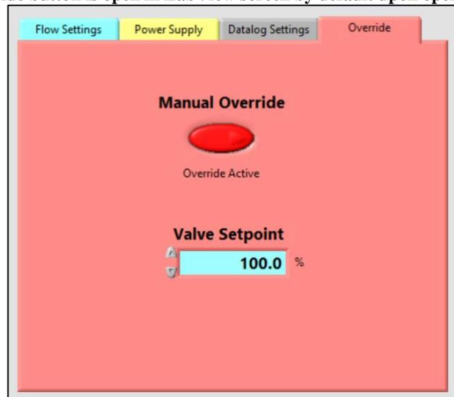
Figure 7. Manual Override button closed manually before SWP testing is started.
