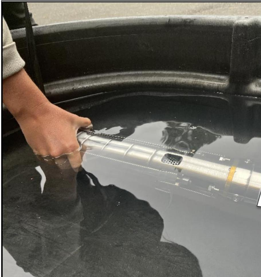
**Figure 18. Submersible pump with its intake screen fully under water.**
