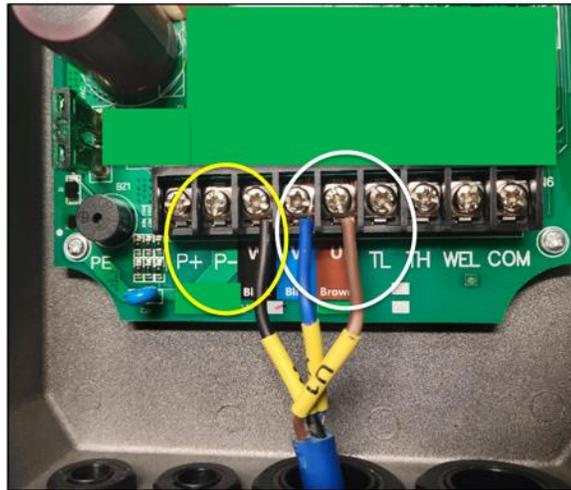
**Figure 19. Screw terminals for PV input and for SWP power output within external controller.**
