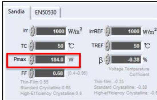
**Figure 17.** Pmax in the Chroma software should be Pmax at TMOT determined in the *IrradianceData* spreadsheet.
