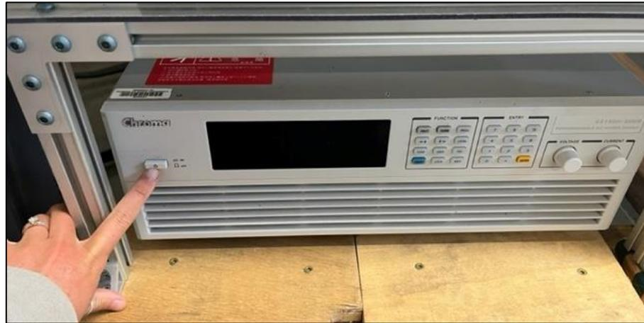
**Figure 11. The Chroma unit OFF has a blank screen- press the button on the left of the screen to turn the unit on.**
