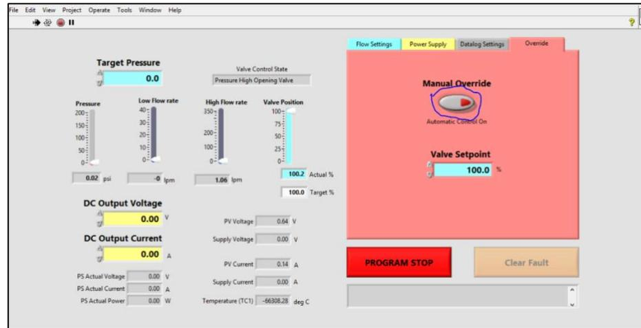
Figure 6. Manual Override button is open in LabView screen by default upon opening the program.
