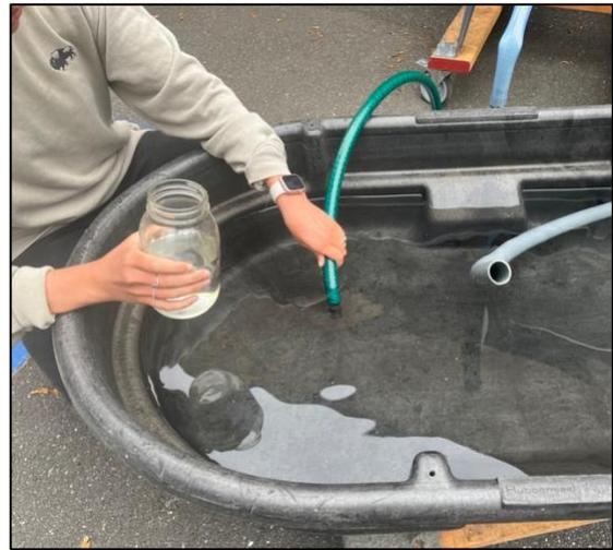
**Figure 2. Creating suction by immediately submerging the pump's inlet hose under the source water after it begins to develop some suction.**
