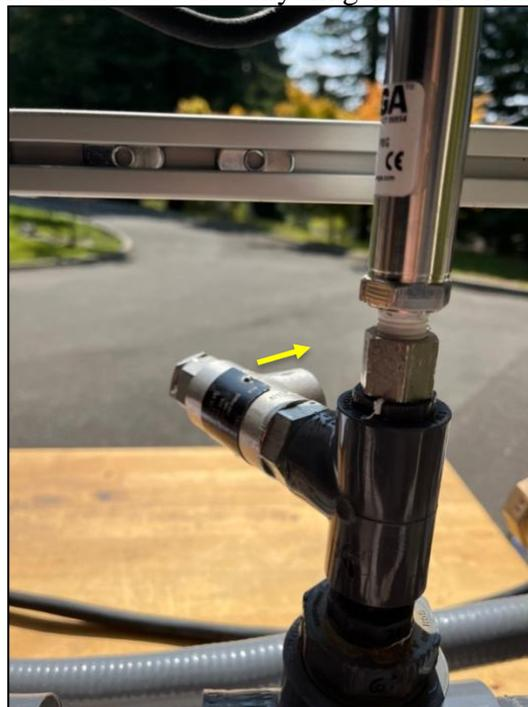
**Figure 3. High pressure safety valve- output facing in a direction outward from the electrical equipment.**
