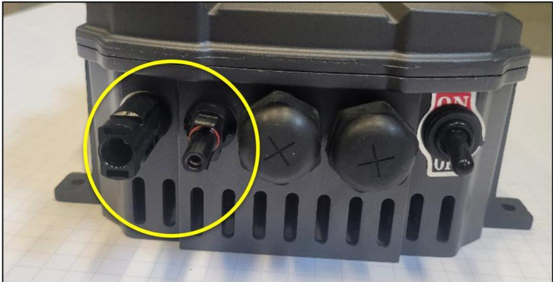
**Figure 22. MC4 connectors for PV input of this external controller.**
