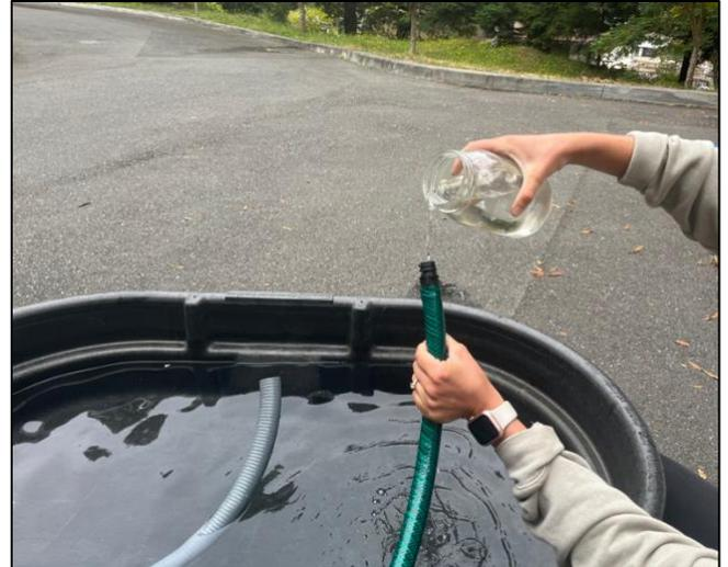
**Figure 1. Priming the surface pump by pouring water down it's intake hose.**
