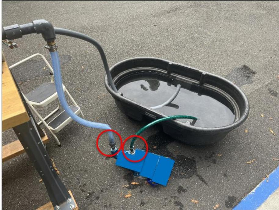
**Figure 17. surface pump needing PVC adapters and hosing for both its inlet and outlet.**
