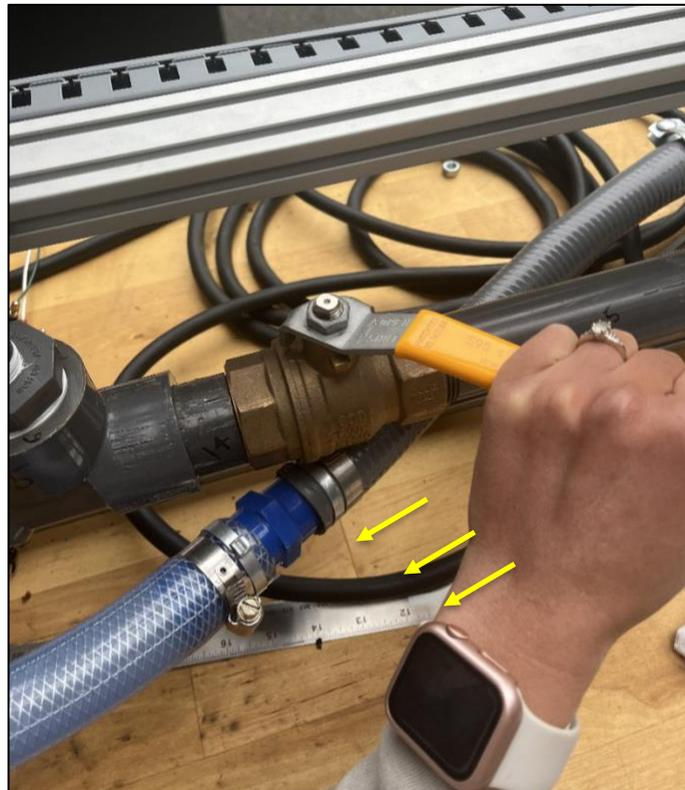
**Figure 27. Slowly closing the high flow ball valve.**
