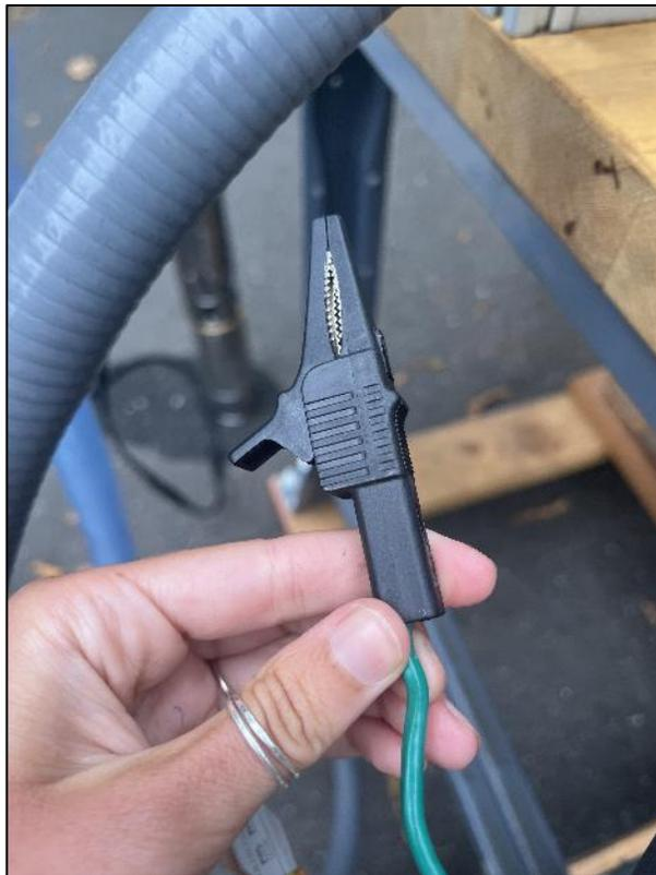
**Figure 14. Alligator grounding adapter with grounding lead on other side.**
