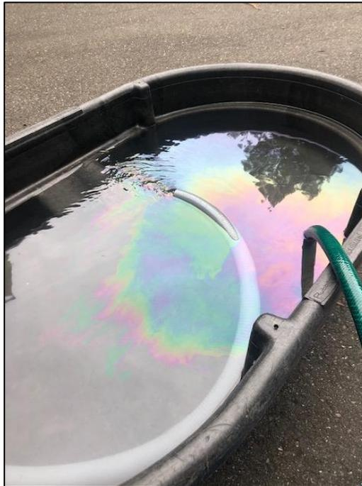
**Figure 5. Oil leaked from a SWP in the source water during testing.**
