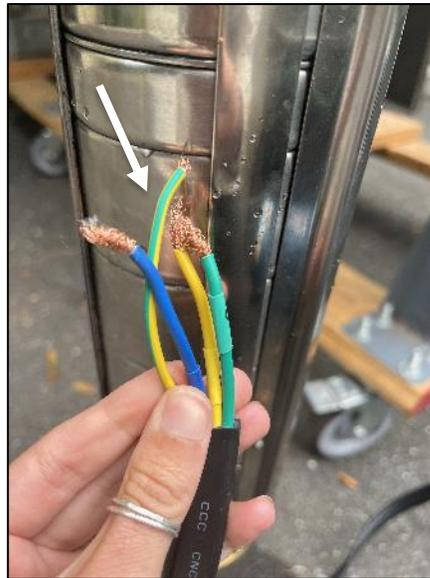
**Figure 12. SWP input power leads, with a grounding lead that is yellow with a green stripe (pointed at by a white arrow)**
