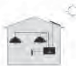
Solar Home System
