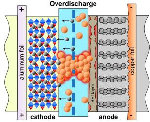
Figure 3. Overdischarge damages the copper anode
