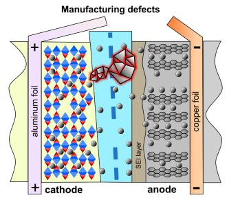
Figure 7. Manufacturing defects can take many forms and pose a serious risk to Li-ion based products
