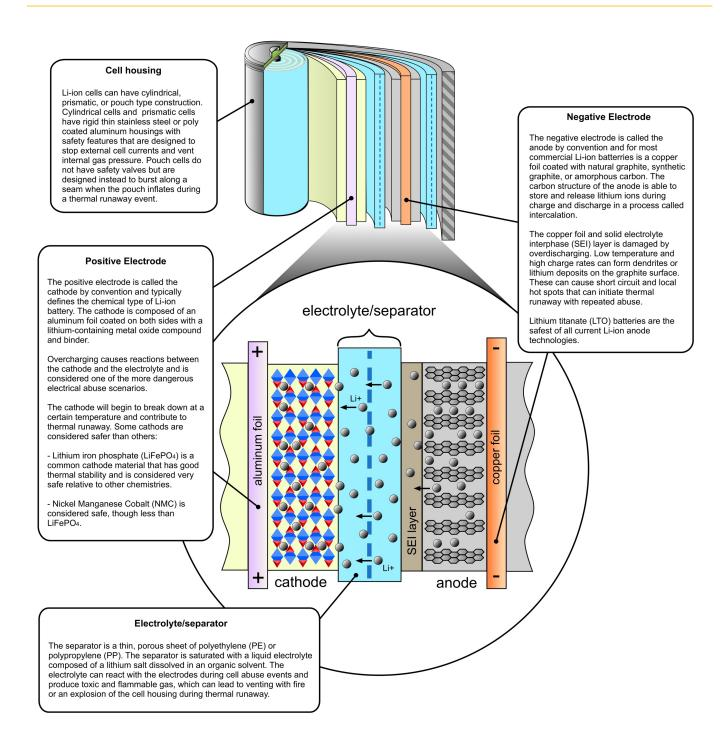
FIGURE 1. A SIMPLIFIED DIAGRAM OF AN 18650 LITHIUM IRON PHOSPHATE (LIFEPO4) CYLINDRICAL CELL BATTERY DEPICTING THE PRIMARY FUNCTIONAL ELEMENTS: CATHODE (POSITIVE ELECTRODE), ANODE (NEGATIVE ELECTRODE), AND ELECTROLYTE/SEPARATOR.
