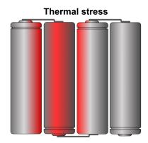
Figure 6. Thermal runaway can spread though the battery pack
