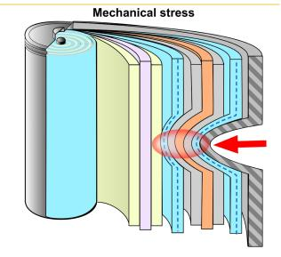
Figure 5. Mechanical stress damages internal layers
