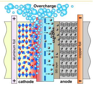
Figure 2. Overcharge releases heat and gas
