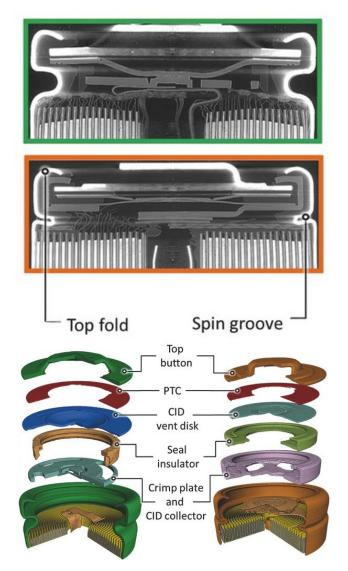
Figure 8. X-ray images and component drawings of two commercial Li-ion 18650 cylindrical cells.
