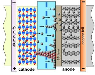
Figure 4. Low temp/high rate charging forms dendrites
