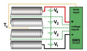
Figure 10. BMS schematic for a 4-series cell battery pack. In this example, the individual cells and the battery pack temperature are monitored. Advanced BMS topologies also include individual cell control and balancing, as well as multiple temperature monitoring inputs.
