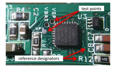
Figure 2. circuit board silkscreen labels
