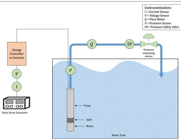
Figure 1: Test station diagram
