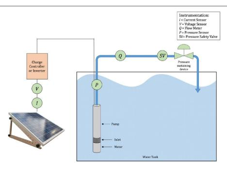
Figure 5: Alternative Test Set-Up
