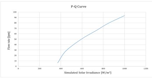
2. Graph this irradiance-flow curve based off of the equation determined in the previous step (Figure 3).
