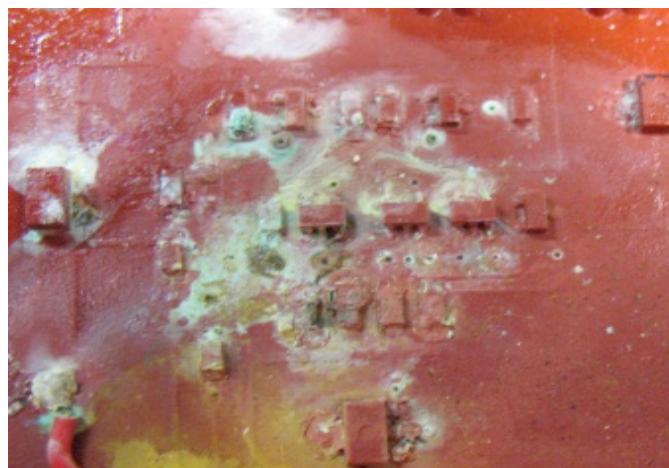
Figure 12. Corrosive failure on a coated PCB
