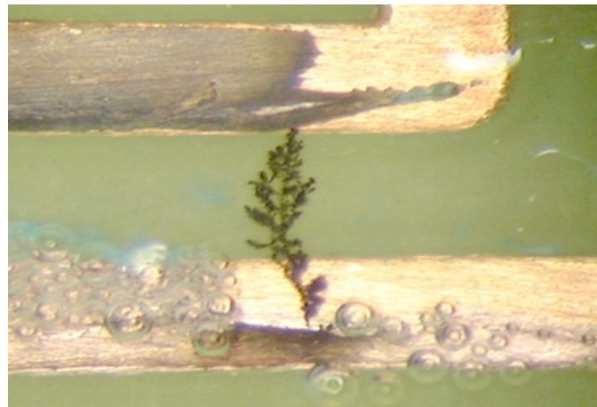
Figure 6. A conductive dendrite short circuit underneath conformal coating.
