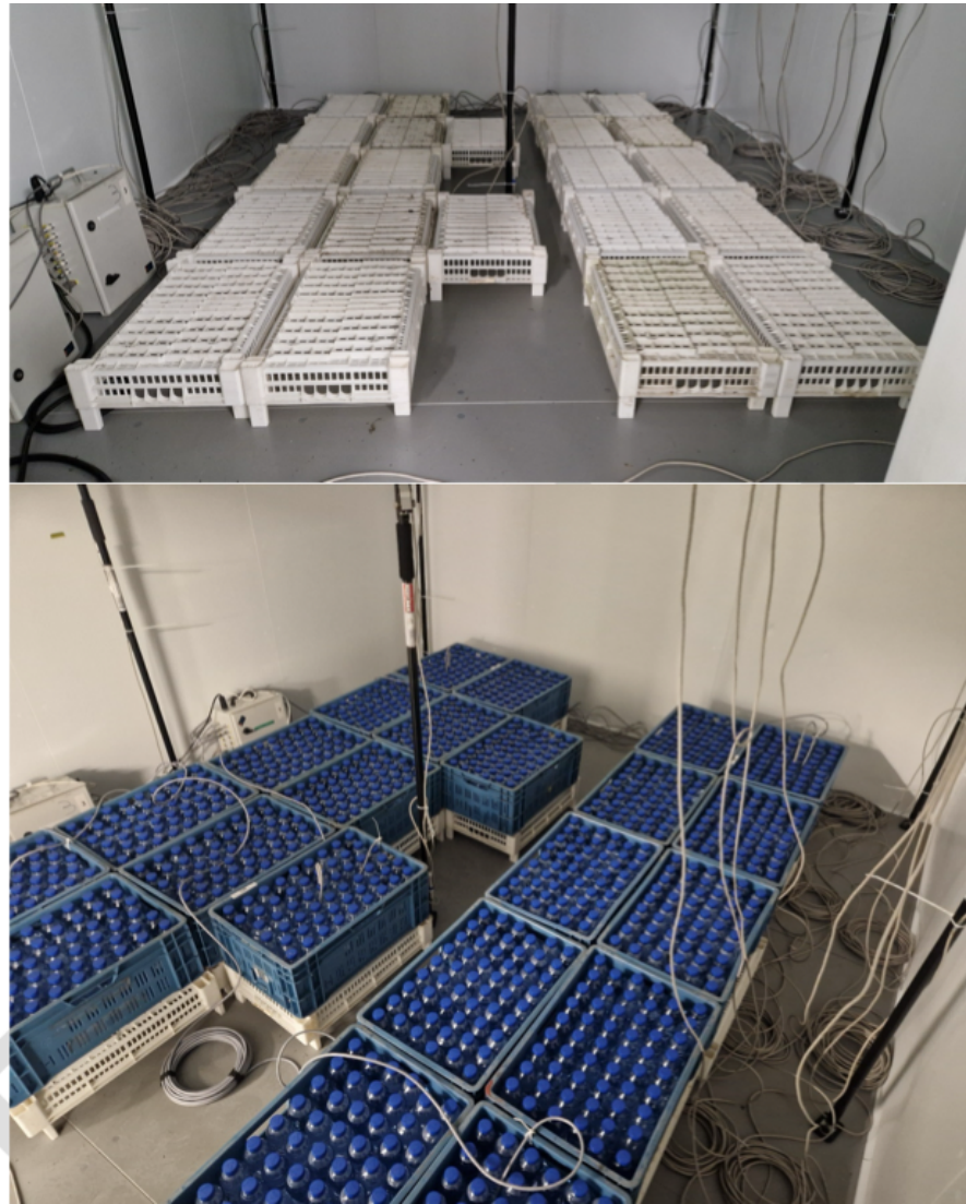
Figure 4. Example stacking of crates of dummy load water bottles in a WICR. Top image: upturned crates on which the dummy load is subsequently placed to allow air flow under dummy load; bottom image: dummy load of crated water bottles in place.
