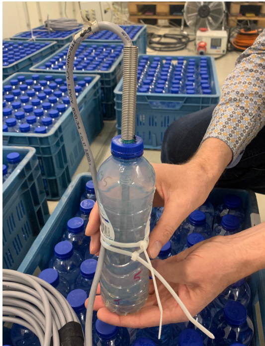
Figure 2. Example M-bottle, with its temperature sensor that is mechanically held at the geometric centre of the bottle.
